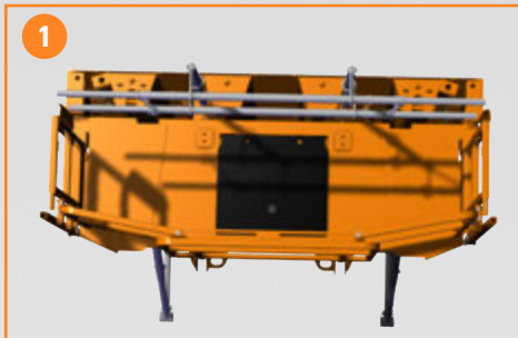
Safety guardrails around the concreting platform.
